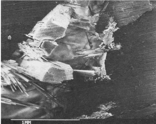
Fig. 11. Combined tensile and interlaminar shear-type fracture of short-beam plane specimens cut from the thin polyester laminate samples.
